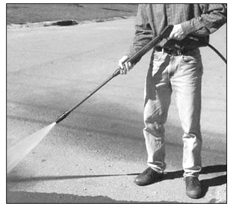
Figure 15 - Optimum angle to cleaning surface
